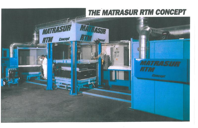
This low pressure, semi-automatic, cyclical production process for the manufacture of parts using composite materials utilizes the combination of MATRASUR Composites vast experience and the very latest technology.
