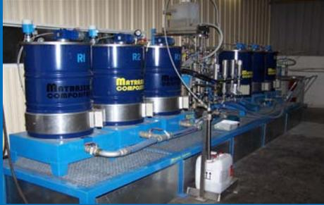
Continuous material dispensing machine for robot 11 axes
