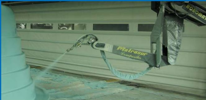
Multi-colour gelcoat spray-up at around 6 m<sup>2</sup>/min
