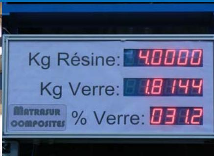
Simultaneous spray-up of resin & fibreglass, at 12 kg/min
